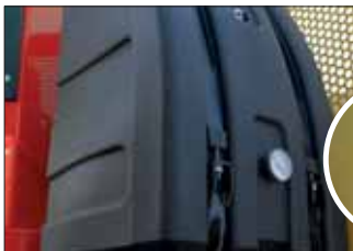
High volume oil tank made in sandwich-structured materials.
